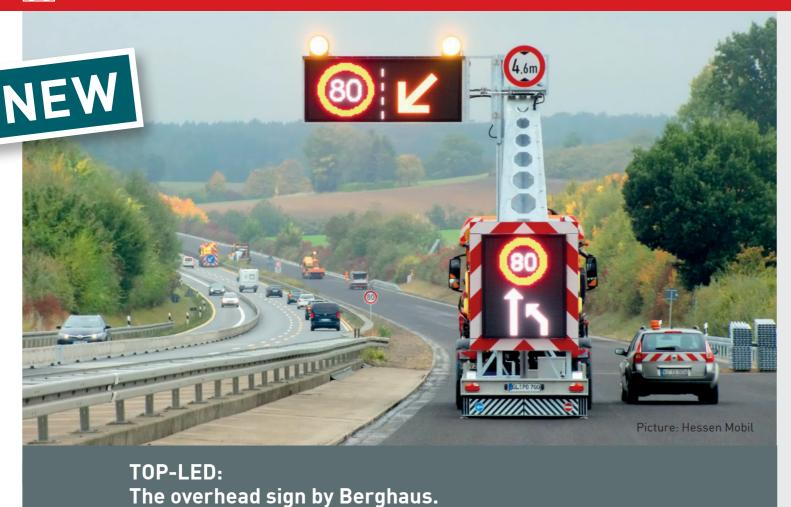
The mobile overhead signs of the "Berghaus TOP-LED" mobile LED prewarner with projecting arm are bright and clear with LED technology at a height of six metres above the carriageway, actively drawing attention to the approaching hazard.
